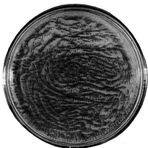
Fig. 4. Pattern in a Petri dish filled to a height 3.29 mm with a solution containing 0.5 M NaOH, 0.1 M D-glucose, 0.1 ml of 1% toluidine blue per 20 ml of solution, 240 s after the start of the experiment.
